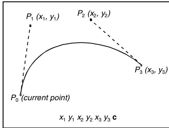
Once these four points are specified, the cubic Bézier curve  $R(t)$  is generated by varying the parameter  $t$  from 0 to 1 in the following equation:
